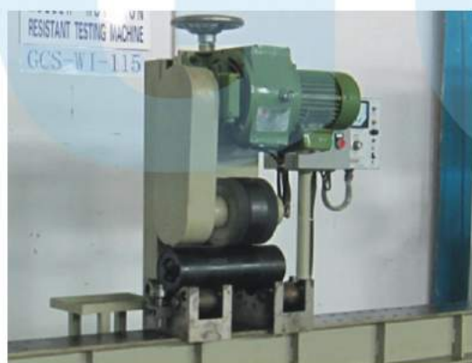
ROLLER ROTATION RESISTANT TESTING MACHINE
