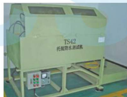
WATER-RESISTANT ROLLER TESTING MACHINE
