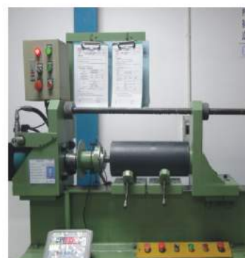
ROLLER SHAFT ANGLE LOADING TESTING MACHINE
